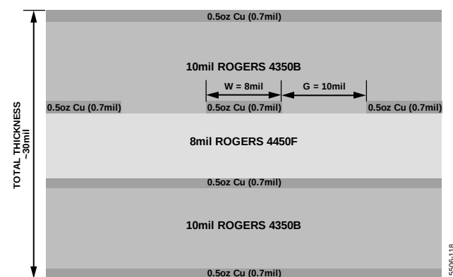
Figure 19. Evaluation Board Cross Sectional View
